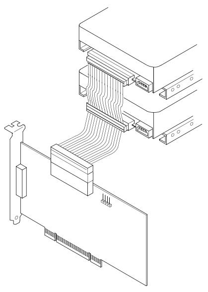
Most PC cabinets are designed with a front panel LED. You may connect the LED cable to connector J4 on the host adapter, as shown in Figure 2.8. This causes the front panel LED to light when there is activity on the SCSI bus.
